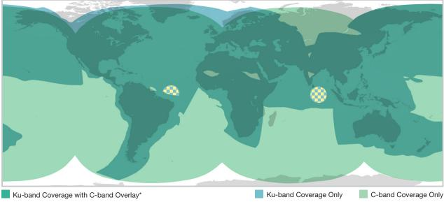
\* The TracPhone V7, V3P and V3 are 2-axis, stabilized antennas that do not provide coverage in areas where the satellite is directly overhead as shown in the hatched areas above
