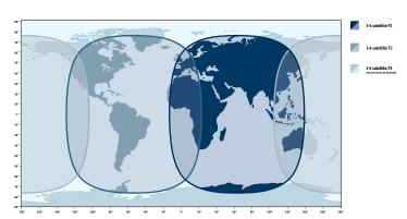
The satellites are placed in geostationary orbit 36,000 kilometers (22,000 miles) above the Atlantic, Indian and Pacific Oceans respectively.
