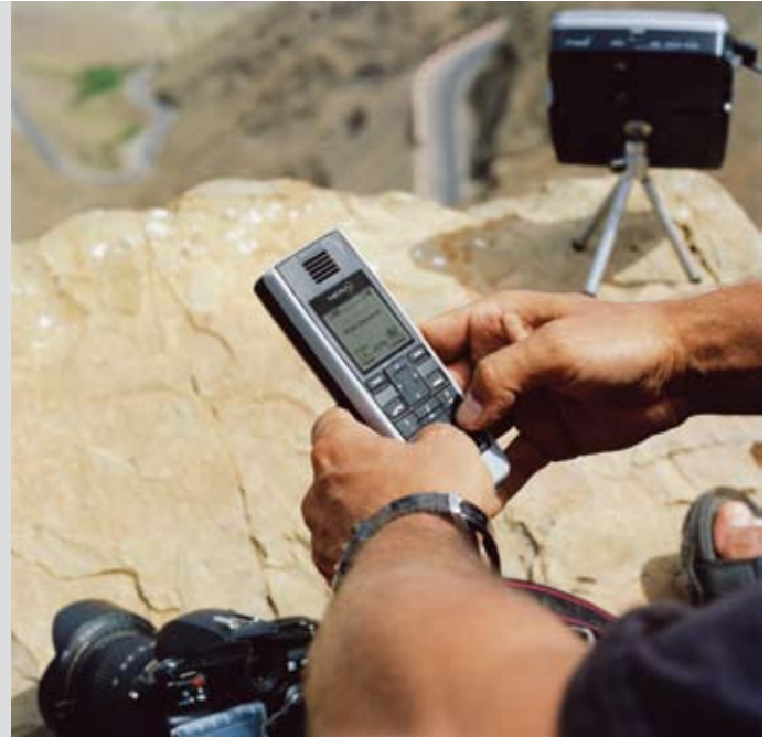
Configuring and controlling the Nera WorldPro directly from the handset.
