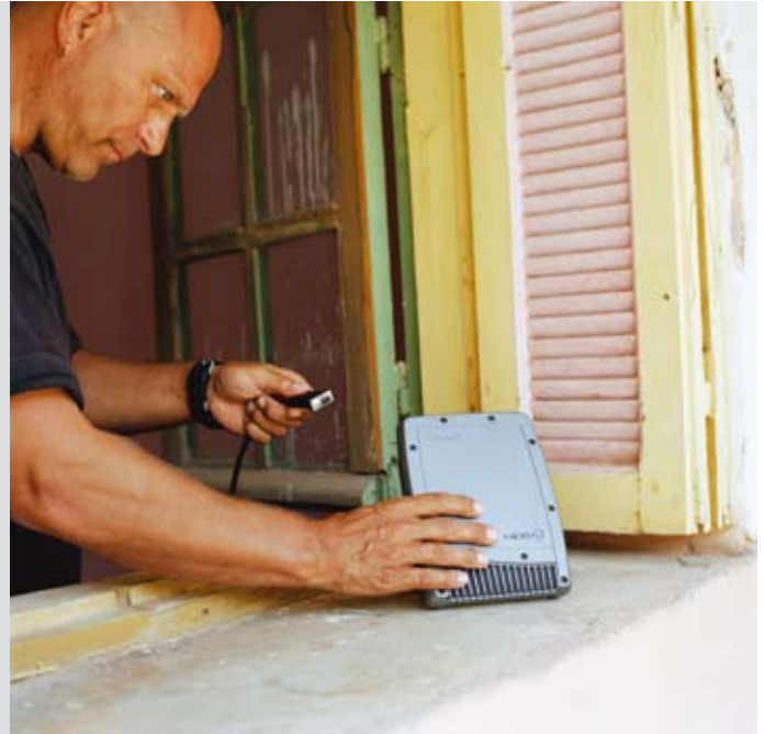
Connecting Antenna Unit of the Nera WorldPro for indoor use.
