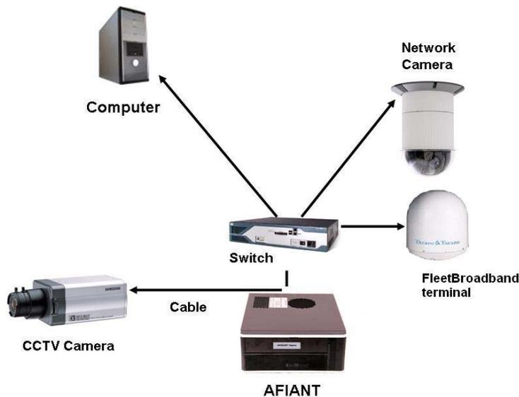
The diagram above shows a simple installation of an AFIANT hybrid. In this example the FleetBroadband Terminal is connected to the network switch, as is the network camera. The CCTV camera is connected directly to the AFIANT hybrid. The computer in this case is a local monitoring and is therefore connected to the switch also. For remote monitoring you would use any computer which had a connection to the internet.
