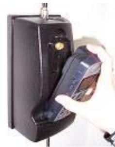
**IMPORTANT:** If the Dock cannot sync with the phone, the top LED will keep blinking and the Dock will eventually re-boot itself and try to sync again. When the top LED goes on solid, the phone will remain on and the Dock is ready for use. If the LED keeps blinking and the Dock continues to re-boot, most common problem is poor Iridium signal strength.
