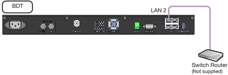
Figure: BDU to Switch Router Cable Connection
