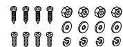
Mounting screws (M5×12 mm), Self-tapping screws (M5×20 mm), Nuts, Flat washers, and Spring washers for mounting the transceiver
