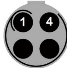
Figure C2 DC connector pin layout (terminal view).
