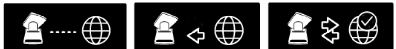
Figure 14 Connection established to modem in the left picture, terminal receive lock in the middle picture, terminal also transmitting with an established internet connection to the right.
