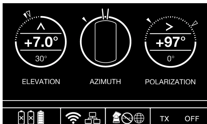
Figure 11 Pointing screen with current pointing values for elevation and polarization, the middle azimuth guidance with signal strength gauge and terminal status bar in the bottom part.
