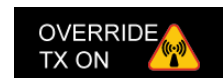
Figure 32 When Override has been enabled the transmit icon changes into this figure
