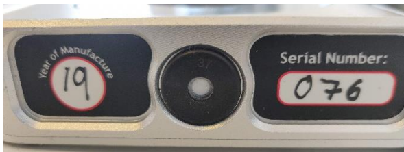
Figure 27 Protective vent on base part of terminal next to the Serial Number.
