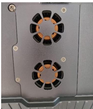
Figure 24 Fans behind fan cover.
