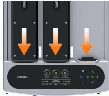
Figure 8 Battery ports are indicated with orange arrows where the right most port charges the battery if the terminal is connected to a power source with the power cable.
