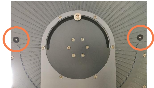
Figure 28 Protective vents on backside of antenna.
