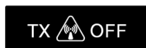
Figure 15 Transmission has been approved by user, pointing or other criteria for transmission not yet fulfilled.
