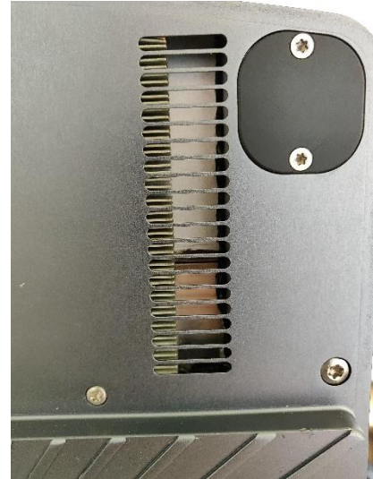
Figure 26 Air exhaust at the backside of antenna.
