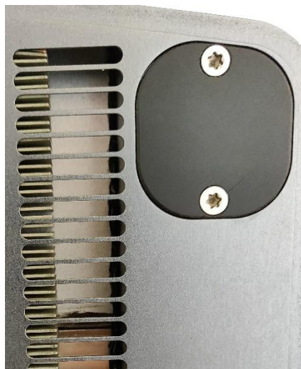
Figure C3a L-band interface, covered.
