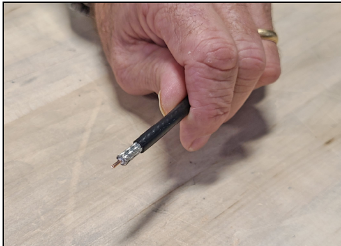
Figure 49: Cable Stripped, Exposing Dielectric
