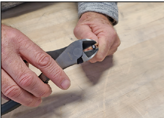
Figure 45: Reshaping the Cable
