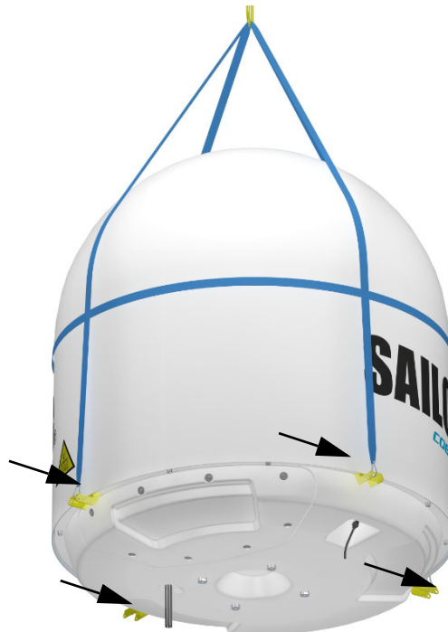
Figure 3-14: ADU installation, webbed sling attached to the 4 lifting brackets
