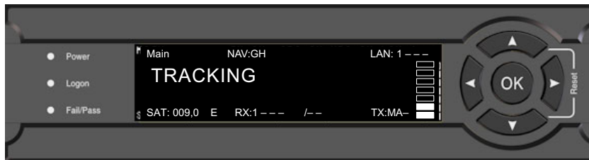
Figure 5-1: ACU: LEDs, display and keypad (detailed, example)
