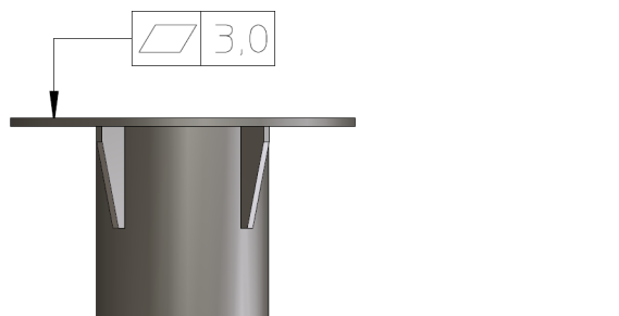
Figure 3-6: ADU mast flange, recommended flatness on the mast mount plateau
