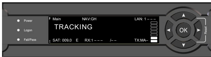
Figure 4-1: ACU: LEDs, display and keypad (detailed, example)
