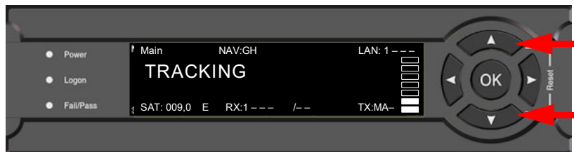
Figure 6-21: Reset the system
