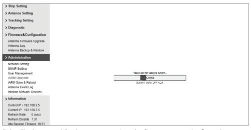
5. It will take around 2 minutes to complete the firmware upgrade. Once the upgrade is completed, the system will reboot automatically.
