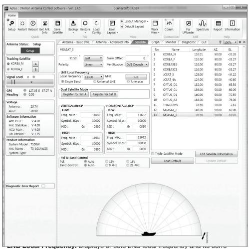
sponding LNB voltage supplied. You may select pre-programmed LNB LO settings from the drop down list. This procedure is same for both the Intellian Global VSAT PLL LNB and any other LNB.
