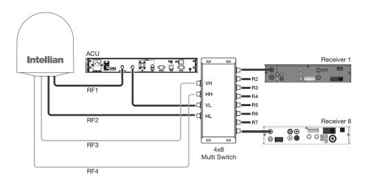
Figure 05. Multi-switch Configuration
