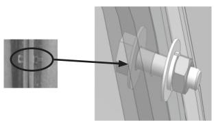
E. Make sure to apply bolt and nut as shown. It is recommended that the max torque be 15Nm.
