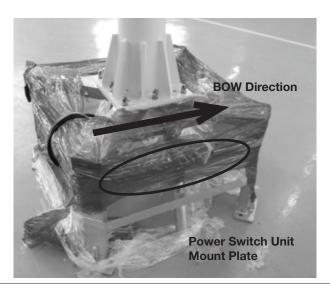
E. Now for the final time, please make sure that the post is attached in accordance with correct bow direction. Power switch unit mount plate should be on the right side when looking from stern to bow of the base assembly.
