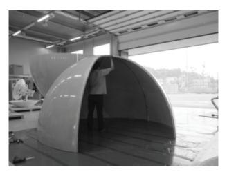
C. Fix the cap in place with a layer of silicon and loosely fasten the M6 bolts but do not tighten them at this time.
