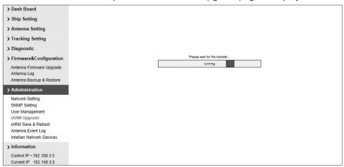
5. It'll take around 2 minutes to complete the firmware upgrade. Once the upgrade is completed, the system will reboot automatically.
