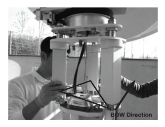
A. Locate the power and RF cables as shown.
