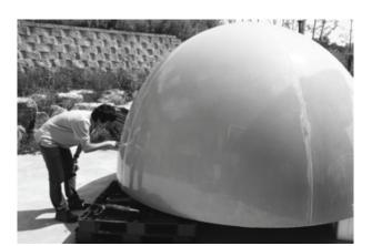
B. Remove excess sealant and smooth to complete the radome top section.
