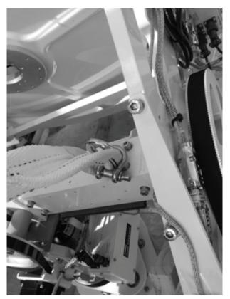
H. Securely hook the lifting straps as shown. (On the both side of the CL arm)
