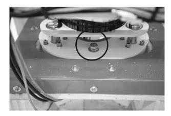
A. Locate the M16 bolts that secure the pedestal assembly to the crate.
