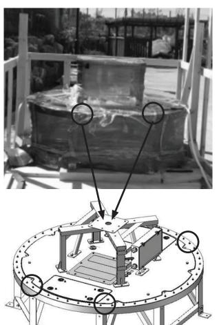
A. Now prepare to attach buckles to base frame in order to lift the base frame from wooden crate.
