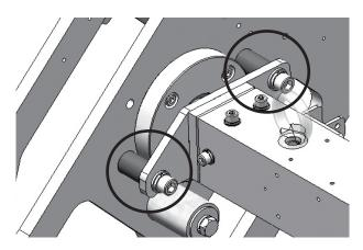
B. Remove the total 4 M12 Hex Bolts securing each side of the EL Arm.
