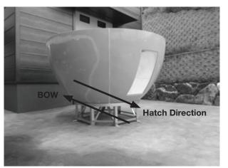
C. Direction of the hatch should be the exactly opposite of Bow direction.
