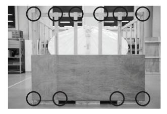
A. Dismantle the wooden assembly of the antenna package using an impact drill.
