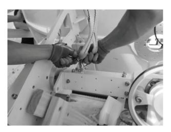
G. Securely hook the lifting straps as shown. (On the both side of the CL arm)
