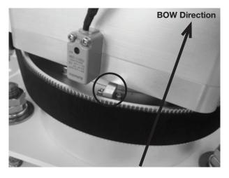
C. The system should be mounted so the AZ sensor is on the stern position of the base assembly.
