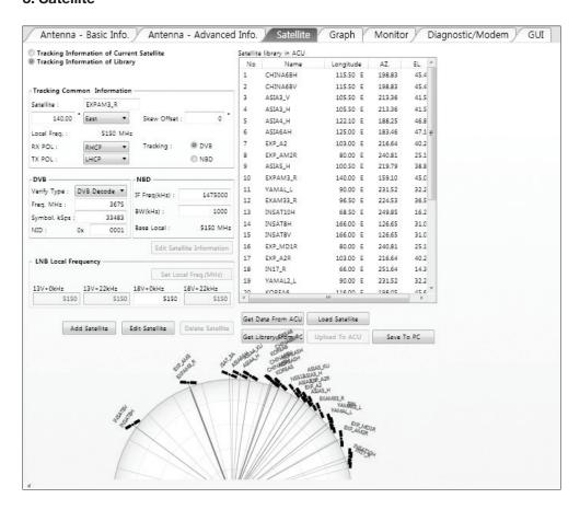
This view provides information on the Satellite's Information, Tracking Common Information, DVB and NBD Tracking Transponder, LNB Local Frequency, and Satellite Library. This view shows a graphic UI of the current satellite that the antenna is pointing at and the satellites that are located at a 180° arc on the horizon with reference to the current position.
