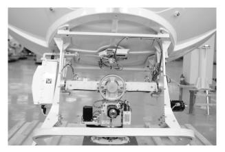
A. Locate the M12 Hex Bolts (4EA) on both sides of the EL Arm.
