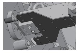
F. Take out all brackets on the rear of the CL ARM by removing M5 flat head bolt (8EA) using an impact drill.
