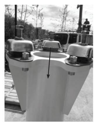
Check to confirm the orientation of the pedestal support with regards to the bow.
