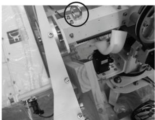
F. 4000mm Lifting straps should be hooked onto the I-bolts as shown left. There should be 2 hooks located on CL arm.
