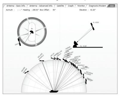
**NOTE:** Based on the satellite EIRP footprint and the size of the antenna, you may not be able to track all the satellites visible in 180° arc.
