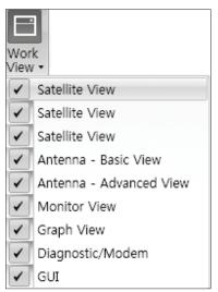
Work View: displays a list of seven pre-constructed Work View Tabs (Satellite View, Antenna Basic View, Antenna Advanced View, Monitor View, Graph View, Diagnostic/Modem View and GUI View and also provides the Activate / Close functionalities for each view tab. Activate the work view tab by ticking the checkbox next to it.
