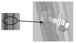
C. Make sure to apply bolt and nut as shown. It is recommended that the max torque be 15Nm.
