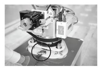
B. Remove the M16 Hex Bolts and Nuts using a wrench as shown left.
