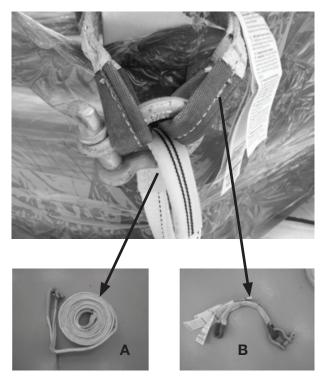
D. Attachment of buckle ropes and lifting ropes should look as shown left.
