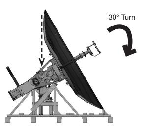
E. As shown in Section C, when the tap is moved, lifting strap can be attached to the CL arm.
