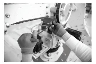
F. Enter the radome hatch and take out 2 brackets under the CL Arm. Remove the M6 Hex bolts to free the CL Arm.
