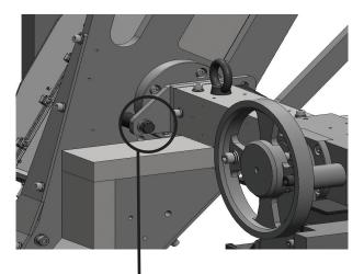
B. This is the initial position of the EL Arm fixture bolt.
