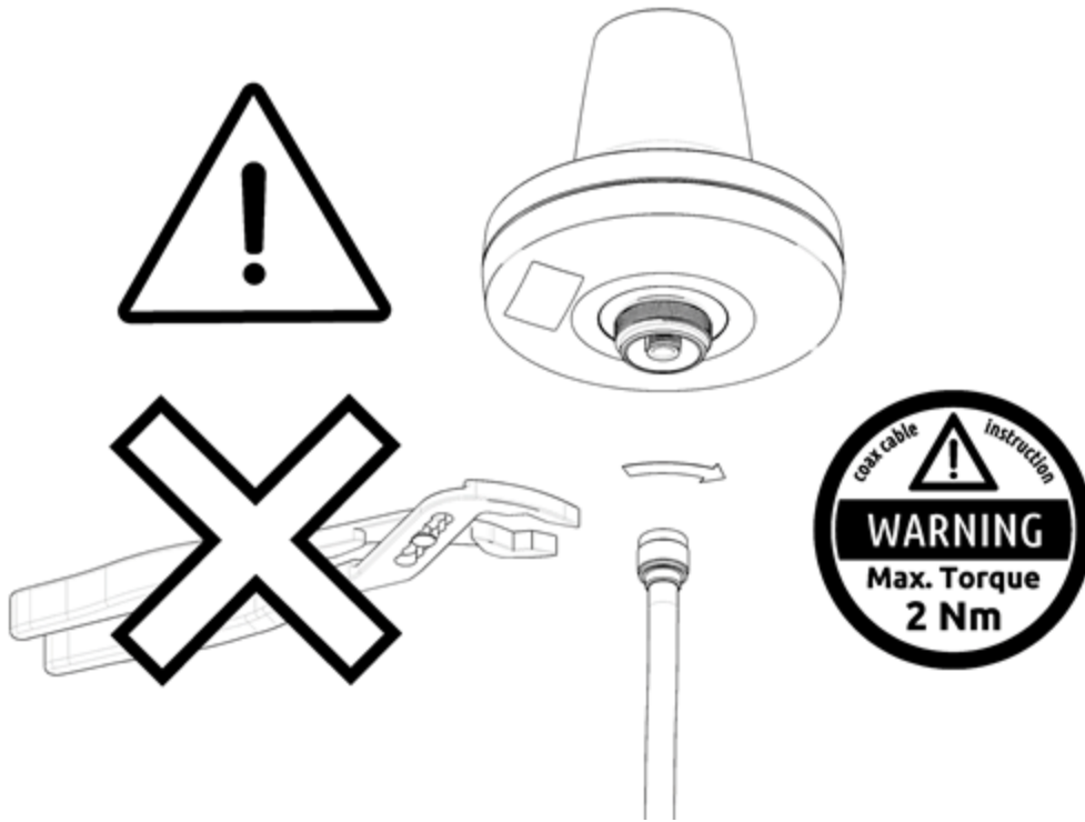
Figure 11: Connecting coaxial cable N-connector to the LT-3130 Antenna Unit
