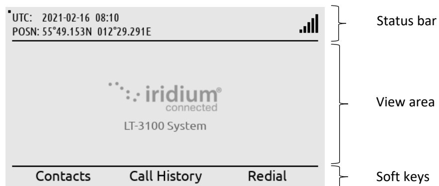
Figure 43: LT-3110 Control Unit - UI display sections
