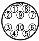
Figure 33: AUX connector pin out
