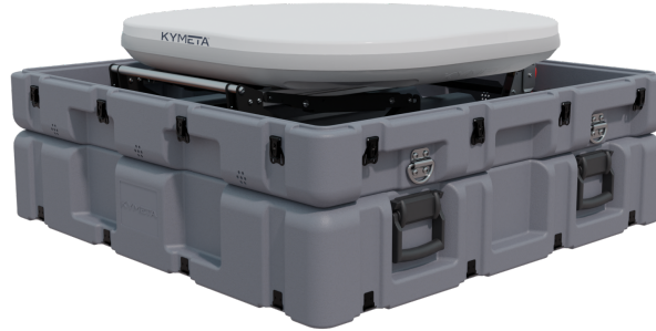
Figure 13: UT with the GO case lid used as a platform
